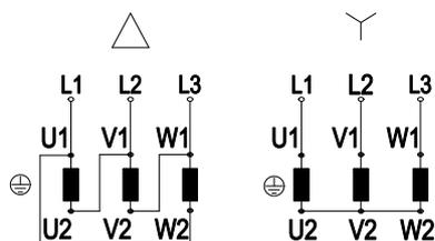
Note: Direction of rotation changes when two phases are reversed
